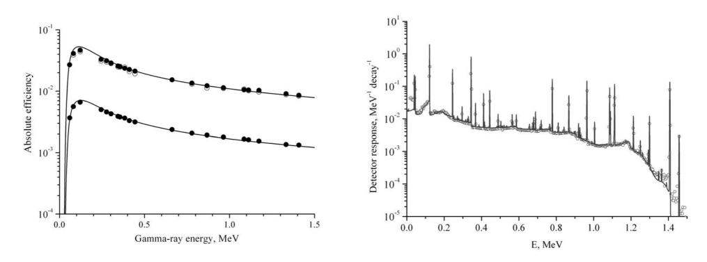
Full Energy Peak efficiency as a function of the photon energy: circles – experimental values, curve – calculated. Two sets of data refer to the source location at 5 cm and 17 cm distances from the detector end cap.
