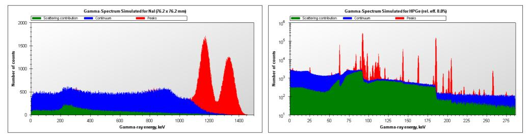
Detector - Nal ( $\emptyset 3'' \times 3''$ ) Source-to-detector distance - 25 cm Measurement time - 1000 s Detector – LEGe (20 mm  $\times$  2800 mm<sup>2</sup>) Source-to-detector distance – 25 mm Filter – 0.5 mm Sn Measurement time - 10<sup>5</sup> s
