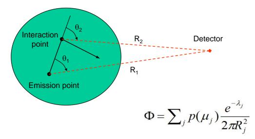
In the **Point Detector** approach the tally is scored, first, when particles emitted from the source, and, then, after each interaction of primary particles, by calculating the probability for all secondary particles to be emitted or scattered directly to the detector.
